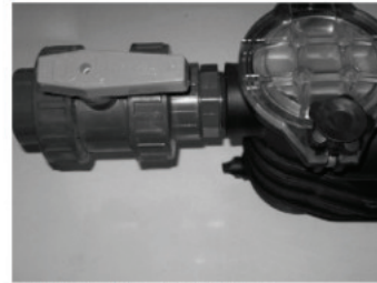
Starting up only with open valves
