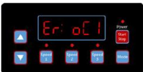
(Diagram 6.8 Fout, foutcode OC1)
