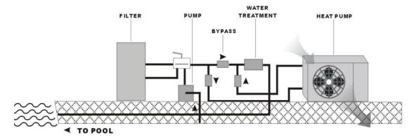
If your installation is equipped of the water treatment with product adductions (e.g. chlorine, brominates, salt...) the by-pass must be installed before the water treatment, with a non-return valve between the by-pass and water treatment.
