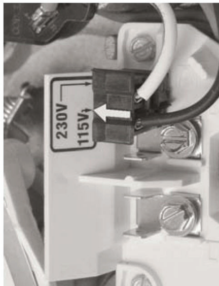
Voltage change plug set for 115 volts
