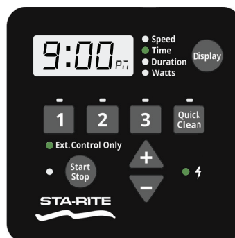
Figure 6: Activating External Control Only
