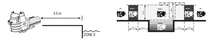
Install the pump in a dry, well-ventilated place. The motor requires the air to circulate freely around it to allow natural ventilation. Check regularly that no objects, leaves or other debris are blocking the motor cooling system.
